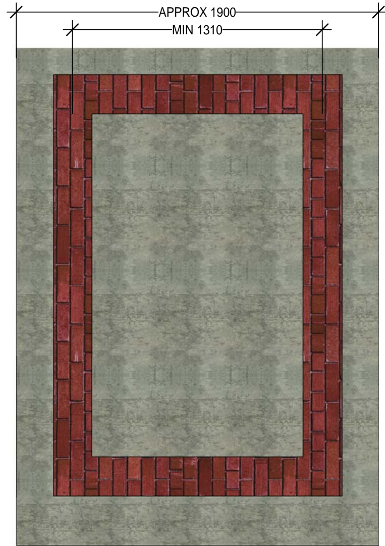
PLAN VIEW OF BASE FOR EXAMPLE VESUVIUS OVEN SCALE AT 1:20 ON A3
