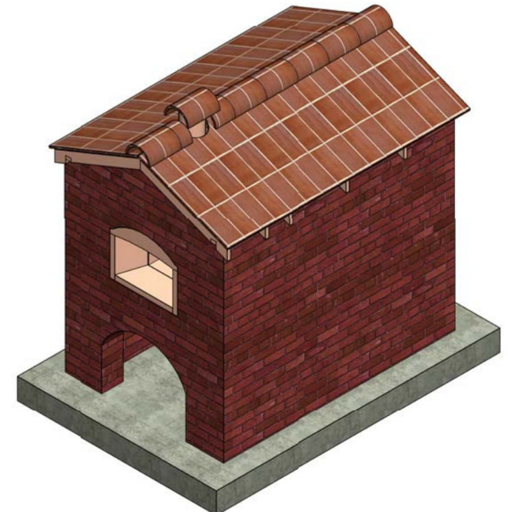
AFFIX ROOF SUBSTRATE ENSURING THAT CHIMNEY PENETRATION IS SEALED WATER TIGHT AND THE CHIMNEY TOP IS COVERED
