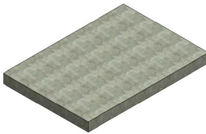
CONSTRUCT CONCRETE FOUNDATION IDEALLY FLUSH WITH GROUND LEVEL AND AT A MINIMUM DEPTH OF 200mm
